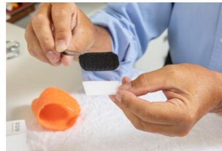
2. Heat up the adhesive glue side of the hook briefly with the heat gun and attach to the Orfit Edging Strip. Trim the corners.
